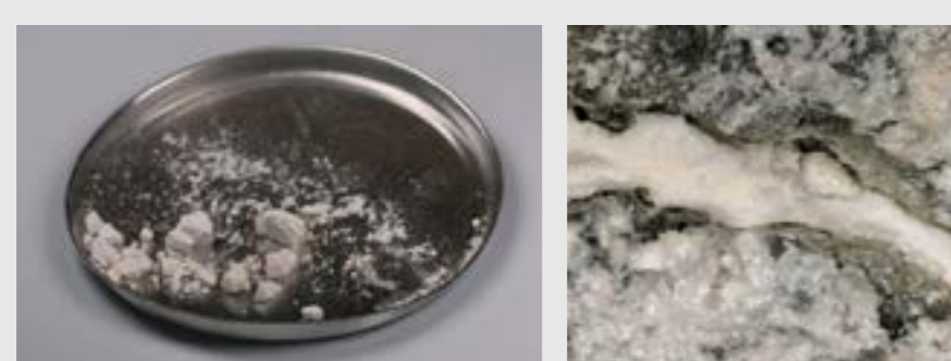
Figure 9a left: Crack healing mechanism by addition of CaO Figure 9b right: Image of the healing process investigated in [9]
