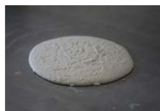
Figure 6: Slump spread testing
