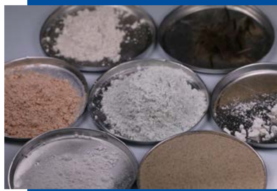
Figure 2: Photographic representation of the used materials in weight representation. Quarzsand, Rutil, Metakaolin, Limestone Powder, basalt microfibers, Calciumoxid aggregates and white cement
